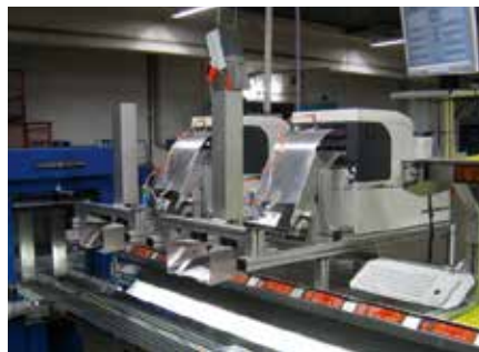
The pusher elevates and pushes the bundle with the wrong weight sideways.
