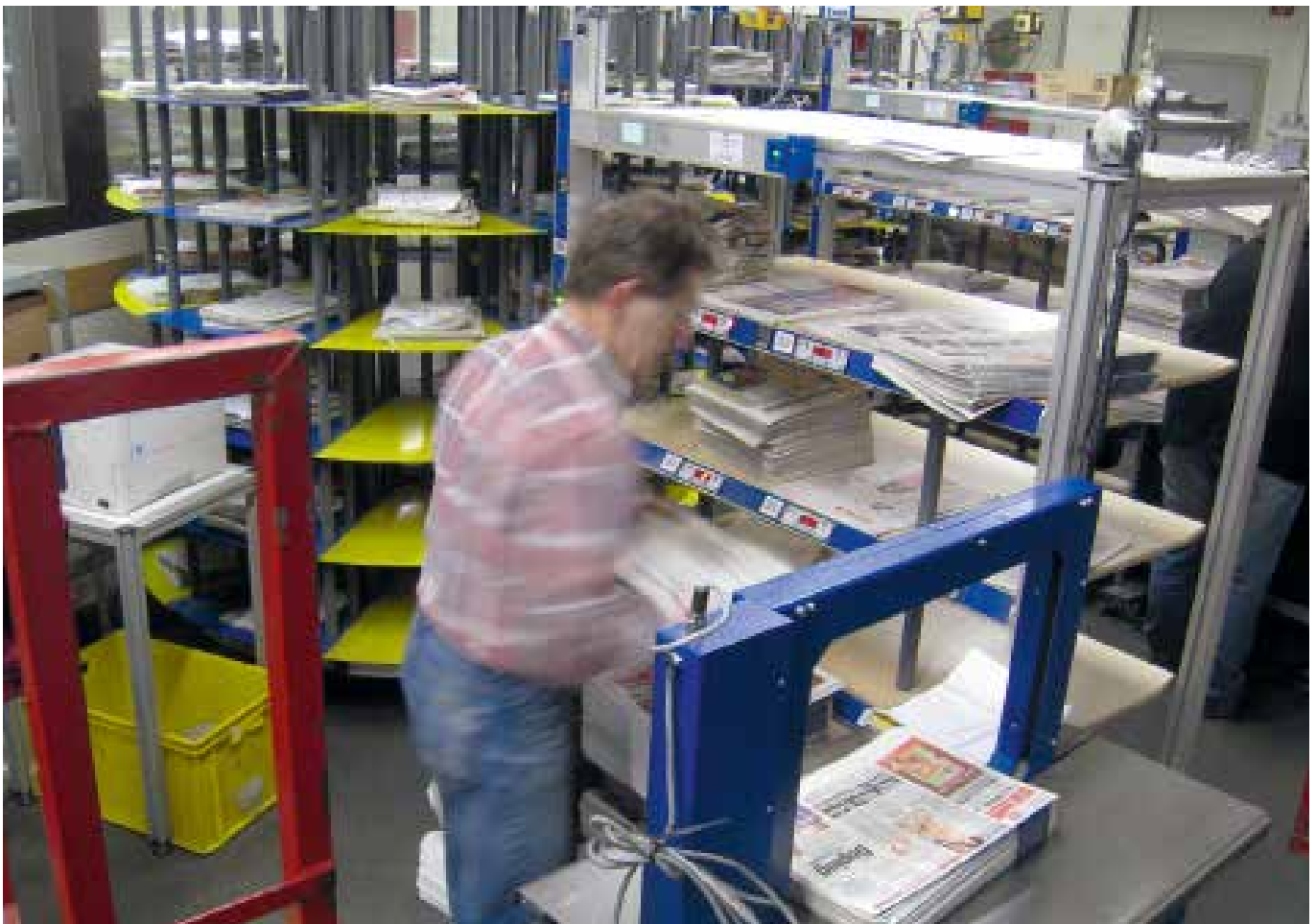
The customer bundles sit in the revolving tower, the titles are in the title trolley sitting behind the title shelf with the displays. The green light of the acknowledgement button indicates the correct package.
