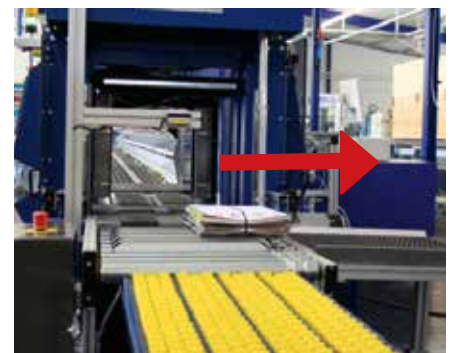
The pusher elevates and pushes the bundle with the wrong weight sideways.
