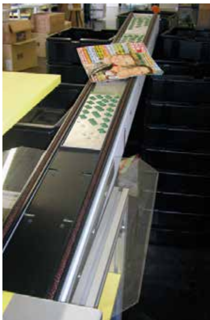
These pictures show the scanning and transportation and the “no read” outlet
