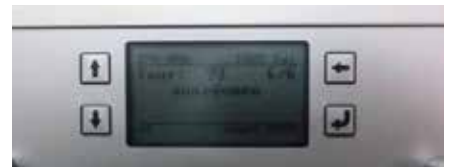
Graphical display with connection to the server, barcode scanner and printer for delivery notes.
