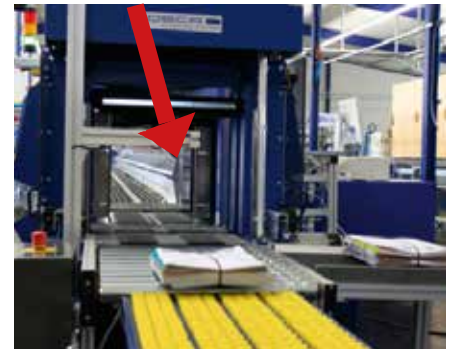
A bundle with the correct weight moves straight on.
